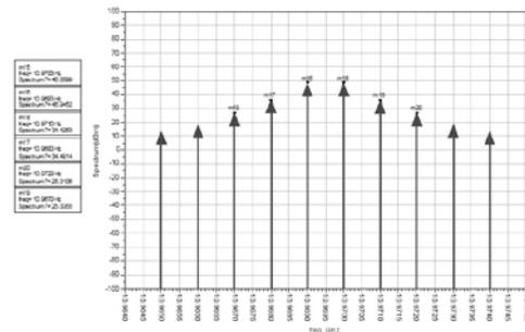
Fig. 8. Spectrum for line of sight link without pre-distortion
