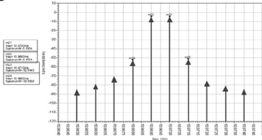
Fig. 7. Spectrum for line of sight link with predistortion
