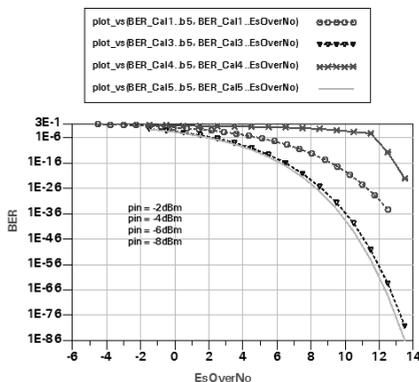
Fig. 12. Eye BER versus  $E_s/N_0$  for three different value of IBO
