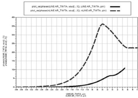
Fig. 6. AM -to- PM characteristic for TWTA
