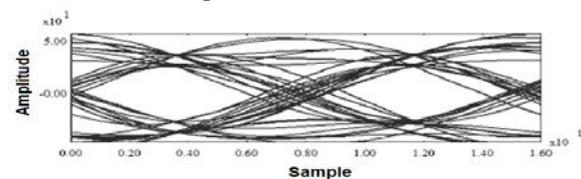
Fig. 10. TK-Eye output in QAM system with pre-distortion
