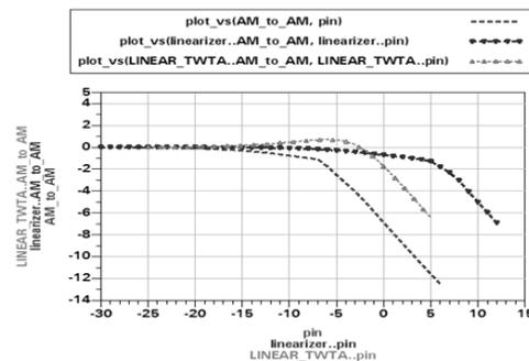
Fig. 5. AM to AM characteristic for TWTA
