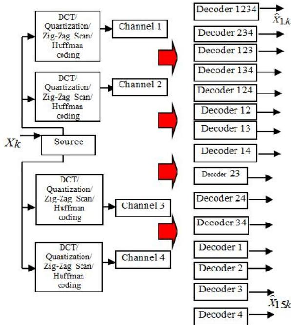
Fig. 4. The structure of four versions coding system based DCT
