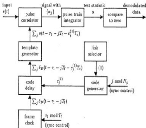
Fig. 3. Structure of receivers in DS-UWB
