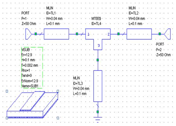
Fig.3. The input matching circuit
