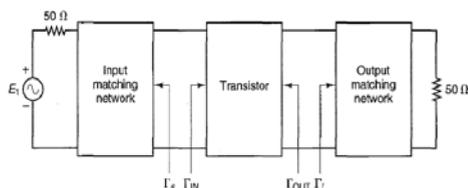
**Fig.1** .Block diagram of a low-noise amplifier [1]
