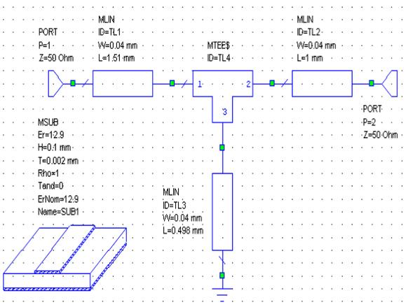
Fig.4. The output matching circuit
