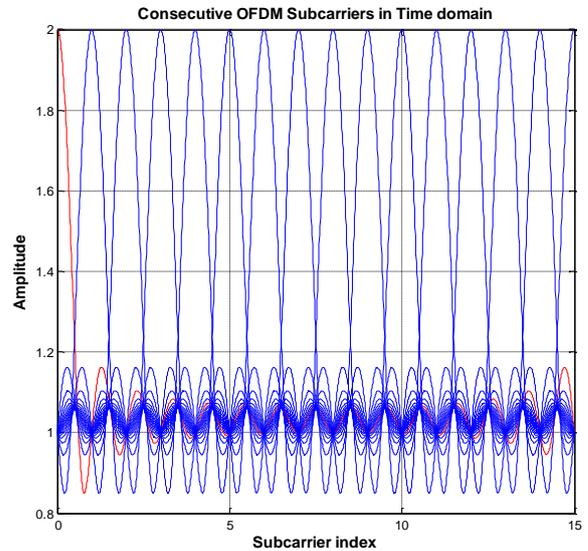
Fig. 3. Computer simulation showing the density of carriers of OFDM signal in time domain
