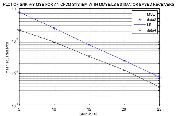
Fig. 5. Computer Simulation showing the SNR performances of the MMSE and LS Channel Estimation Methods on the receiver in a 64-carrier OFDM system.
