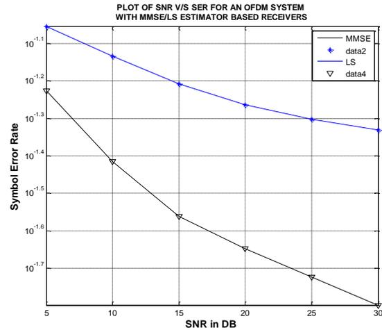
Fig. 4. Computer Simulation showing the SNR performances of MMSE and LS Channel Estimation Methods in OFDM systems on the receiver side.
