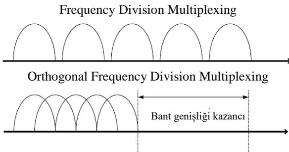
Fig. 2. Bandwidth savings provided by using OFDM.[1]
