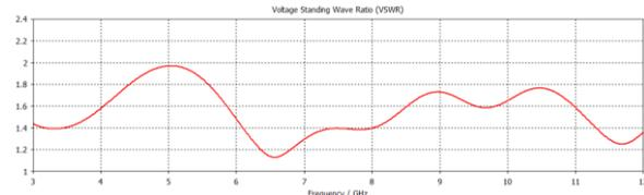
**Fig. 3.** Graphic of Voltage Standing Wave Ratio of Vivaldi antenna.
