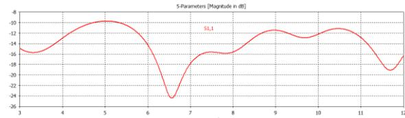
**Fig. 2.** Graphic of S-parameter ( $S_{11}$ ) of Vivaldi antenna.
