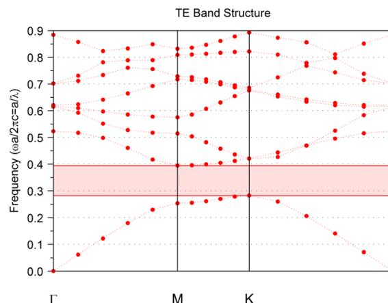
**Fig 1:** The structure of crystal band used for designing an optic filter
