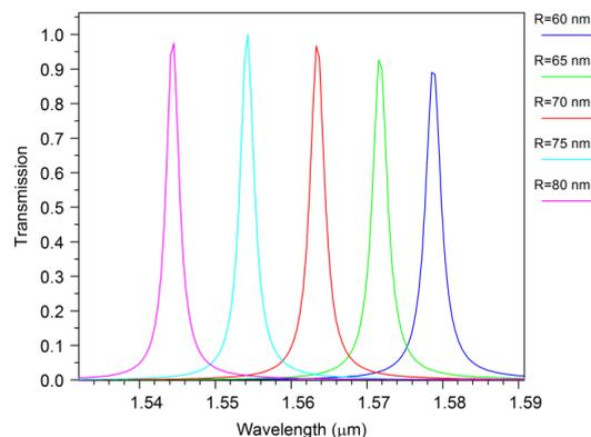
Fig 4: Output spectrum of filter for different amounts of  $R$ .
