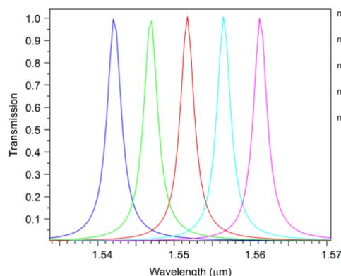
Fig 5: Output spectrum of filter for different amounts
