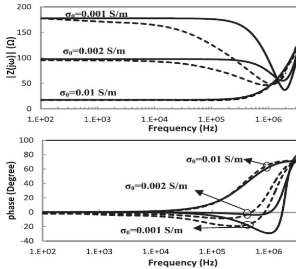
**Fig. 3.** Frequency dependence behavior of the input impedance of grid-grounding system [11].
