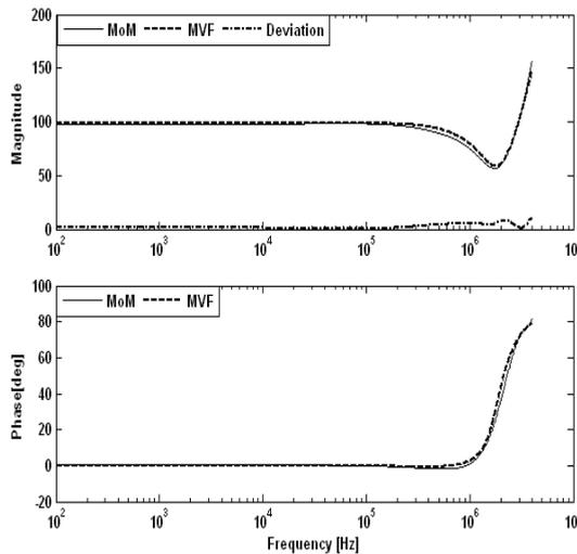
**Fig. 4** Modeled input impedance by the MoM and MVF for  $\sigma_0 = 0.001S/m$
