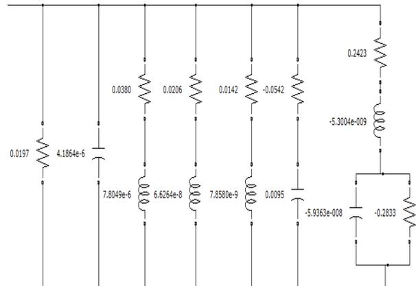
**Fig. 6.** Equivalent circuit of grid-grounding system with considering frequency dependence of soil for  $\sigma_0 = 0.001S/m$
