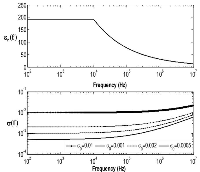
**Fig. 2.** Frequency-dependent behavior of electrical parameters of lossy soil.
