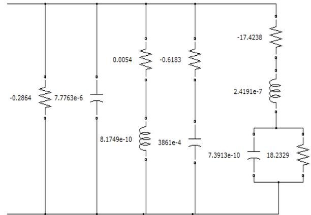
**Fig. 5.** Equivalent circuit of grid-grounding system without considering frequency dependence of soil for  $\sigma_0 = 0.001S/m$
