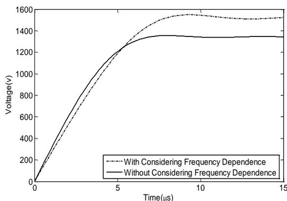
**Fig. 7** lightning-induced voltage of surge arrester with and without considering frequency dependence of electrical parameters of soil.
