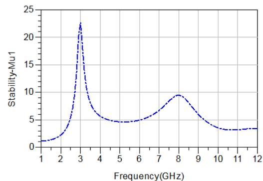
Fig. 8. Stability factor ( $\mu$ ) of proposed UWB LNA.
