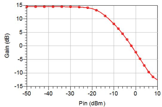
Fig. 6.  $P_{-1\text{ dB}}$  of proposed UWB LNA.
