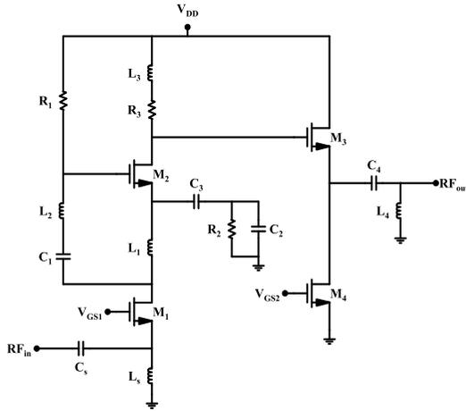
Fig. 1. Proposed high-flat gain LNA.
