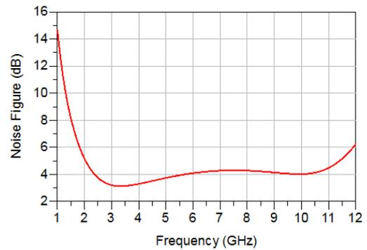
Fig. 5. NF of proposed UWB LNA.
