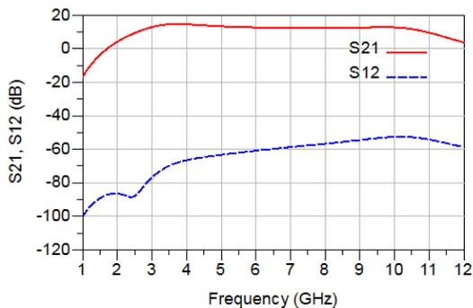
Fig. 4. Power gain and isolation of proposed UWB LNA.
