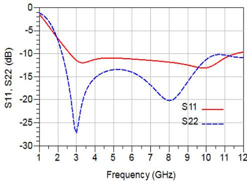
Fig. 2. Input and output reflection coefficients of proposed UWB LNA.
