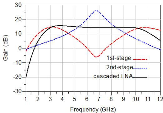
Fig. 3. Simulated  $S_{21}$  of the overall stage and the voltage gain of each stage.
