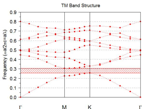
Fig. 2. Structure of 2D photonic crystal band gap for designing two-channel demultiplexer basic filter
