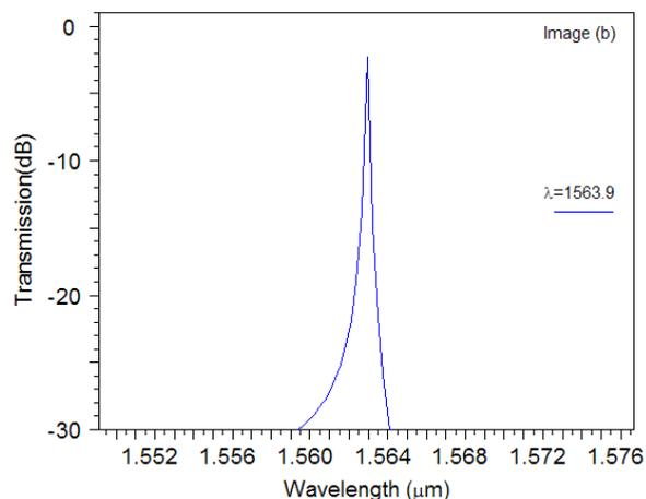
**Fig. 5.** Output spectrum of suggested two-channel demultiplexer basic filter of 2D photonic crystal lattice a) linear scale b) dB scale.
