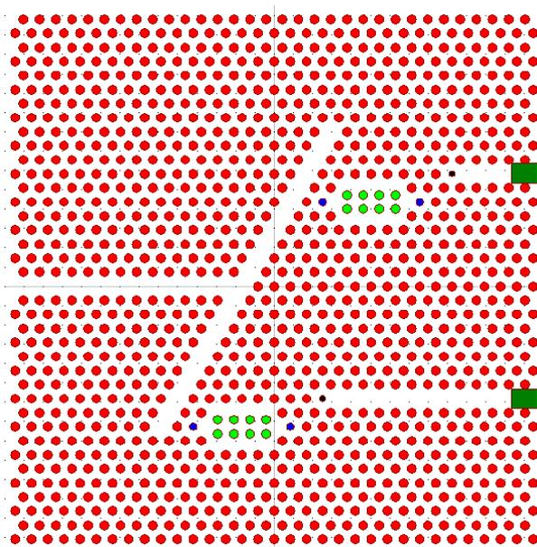
**Fig. 6.** T-shaped two-channel demultiplexer of 2D photonic crystal
