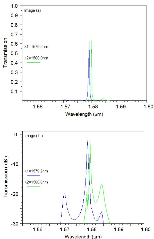
**Fig. 7.** Transfer spectrum of T-shaped two channel demultiplexer of 2D photonic crystal a) linear scale b) dB scale
