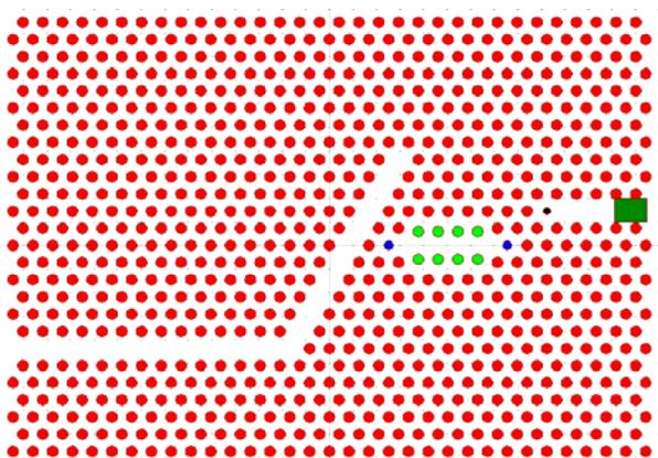
**Fig. 4.** Two-channel demultiplexer basic filter structure of 2D photonic crystal lattice
