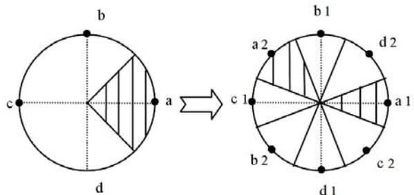
**Fig. 5.** The constellation expansion from QPSK to 8PSK with the map on the real or imaginary axis
