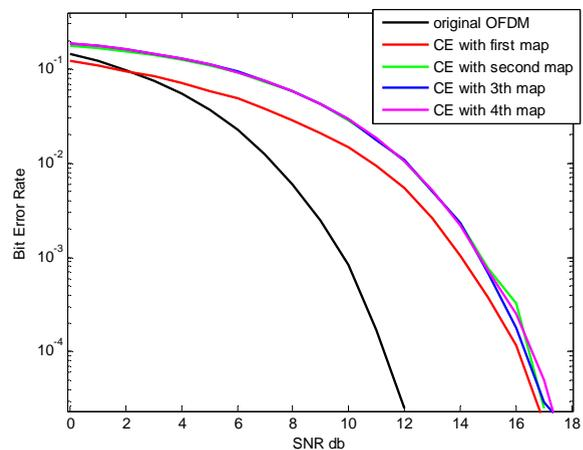
Fig. 7. BER of original OFDM signal, CE method with first, second, 3th and 4th maps
