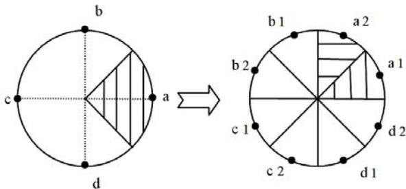
**Fig. 2.** The constellation expansion from QPSK to 8PSK with the map with same sign in real and imaginary part
