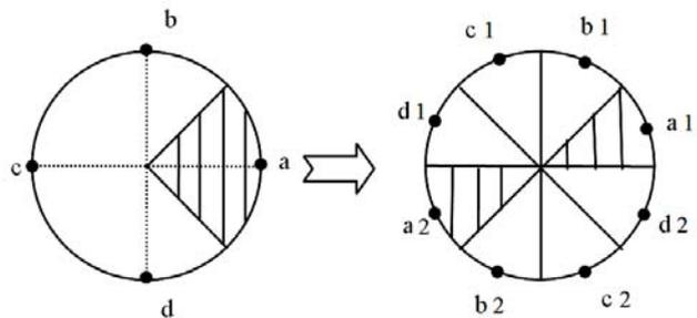
**Fig. 4.** The constellation expansion from QPSK to 8PSK with the map with different sign in real and imaginary part
