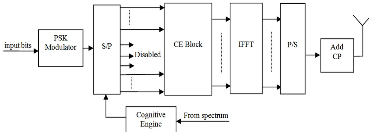
Fig. 1. Block diagram of transmitter for OFDM based CR with using CE method
