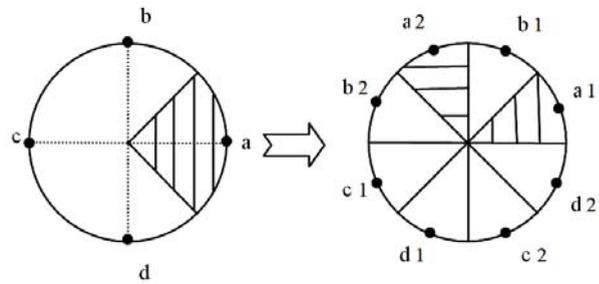
**Fig. 3.** The constellation expansion from QPSK to 8PSK with the map with same sign in real or imaginary part
