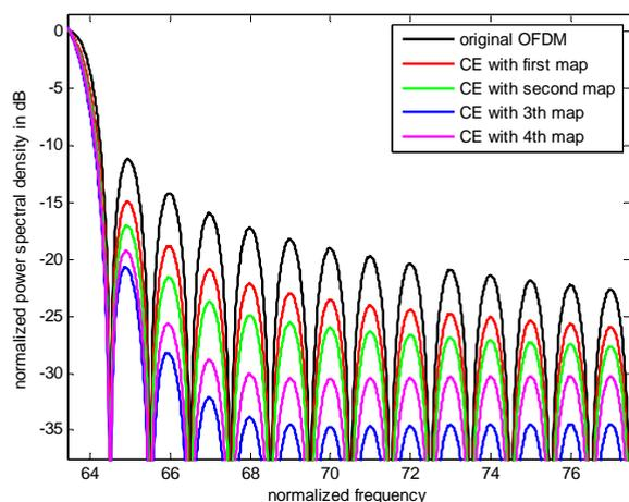
Fig. 6. Power spectrum of original OFDM signal and CE method with first, second, 3th and 4th maps
